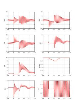
Voltage dip at terminals of 100KW three phase motor driving a pump -
