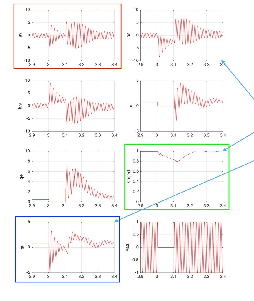
Short circuit at terminals of 100KW three phase motor driving a pump -
