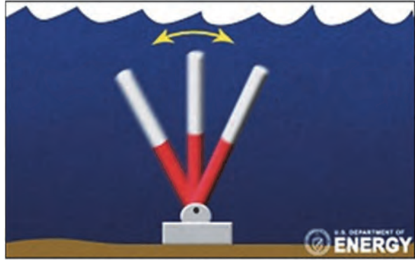
Figure 2-31. Illustration of Oscillating Wave Surge Converter Technology
