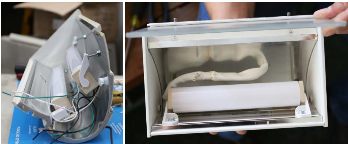
Figure 2. LED Modules in Existing Wall Washer Housings. The left image is a side view of the large wall washer housing with two LED modules and the right image is a front view of the small wall washer housing with one LED module.
