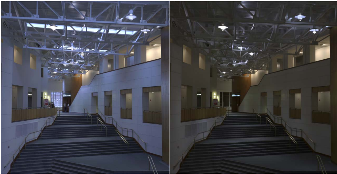
Figure 4. Interior View of the UMD CSPAC Atrium. The wall washers illuminate the hallways that line the atrium during the day (left) and evening (right) as well as some surrounding areas. The brightness of the hallways is faint during the day compared to the daylight washing the main walls of the atrium; however, in the evening these perimeter hallways play a more dominant role in the visual appearance of the space.
