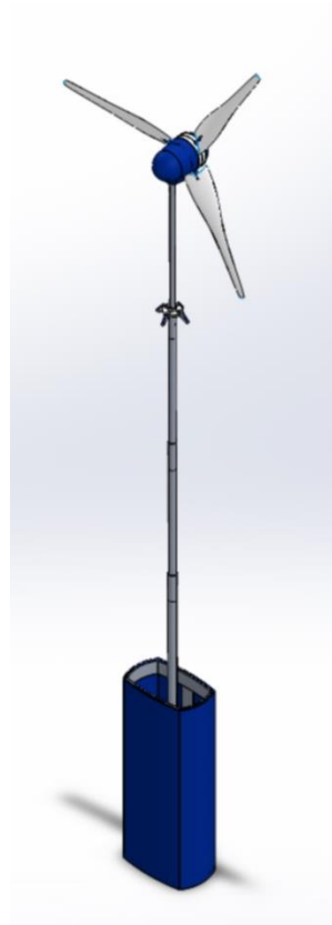
Figure 1: Deployed Market (M152) Turbine (Without Guy Wires Shown)
