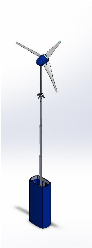
Figure 1: Deployed Market Turbine (Guy Wires Not Shown)
