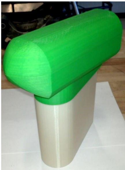
Figure 5: Rapid Prototyped Nacelle
