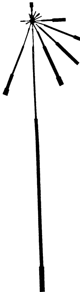
Figure 2.1-2 Wind Rose, AGA Tenneco Platform, Location 27 59N, 93 02W - September 1977.
