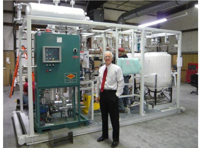
2015 Federal Laboratory Consortium Award Winning Team, 1000 L/day (20 wt% BDAF) system Reliance-PNNL-Genifuel HTL/CHG System
