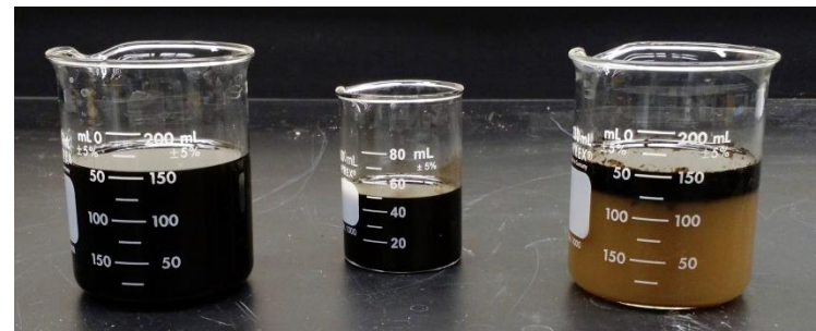
Pilot plant products (l-r): light wood oil, heavy wood oil, light wood oil and water
