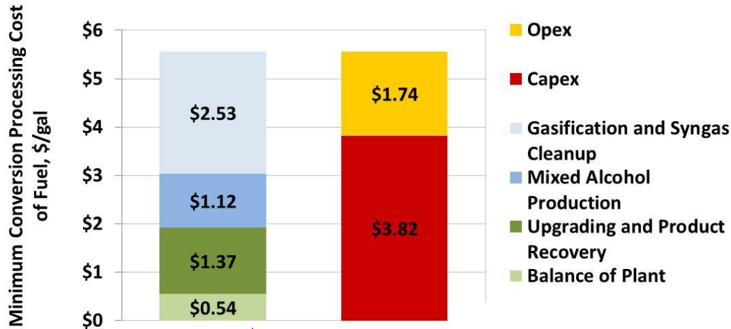
Conversion Contribution (ex feedstock) by Area Gasification to syngas, alcohol synthesis and upgrading
