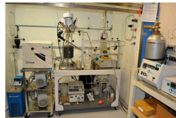
CSTR reactor for carbon coupling reactions with biomass compounds.
