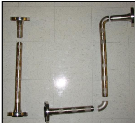
Spool piece fabricated with 6 different alloys and installed in KiOR's operating system
