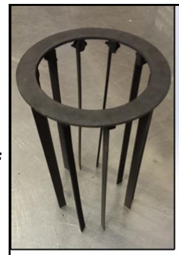
Sample rack with coupons being exposed in freeboard area of ISU's fluidized bed pyrolysis system
