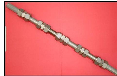
Spool piece fabricated from 6 different alloys and installed in GTI's system
