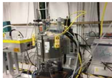
Plug reactor system for conducting operando studies.
