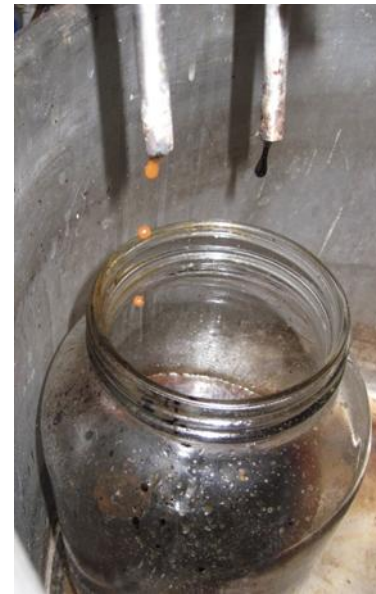
Biocrude /aqueous product separation during continuous product collection. Invention Report
