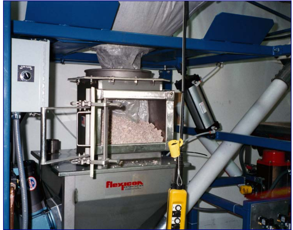
Dried paper mill sludge is fed into the hopper at a biorefinery plant.
