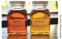
Raw fish oil and fish oil biodiesel from the Unisea plant in Dutch Harbor.
