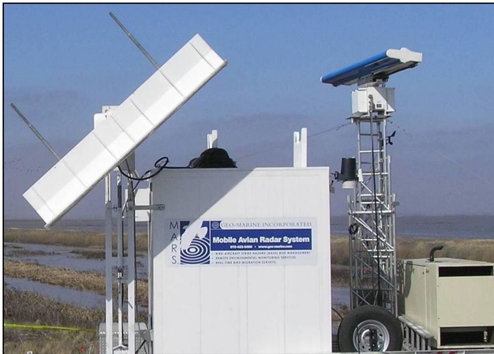
Figure 1. GMI MARS® showing both VerCat (vertically scanning) radar (left) and TracScan (horizontally scanning) radar (right), the computer housing unit, and the generator.
