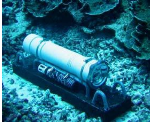
Figure 1. Shallow-water EAR attached to lead anchor. (From Lammers 2010 [spec sheet]).
