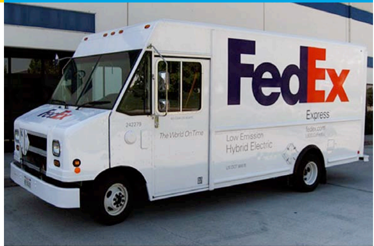
FedEx Express's gasoline hybrid-electric delivery trucks demonstrated lower tailpipe emissions compared with conventional diesel delivery trucks. Courtesy of Sam Snyder, FedEx Express
