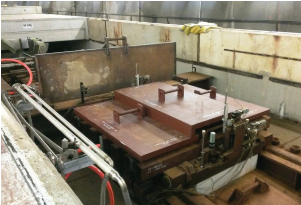
Exhibit 4-8: NuMI Shielding Platform
