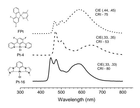
For Pt-16 WOLED, power efficiency exceeds 50 lm/W (no n/p-doping and enhanced outcoupling), CIE (0.33, 0.32), CRI >=80, showing promise for lighting applications.
