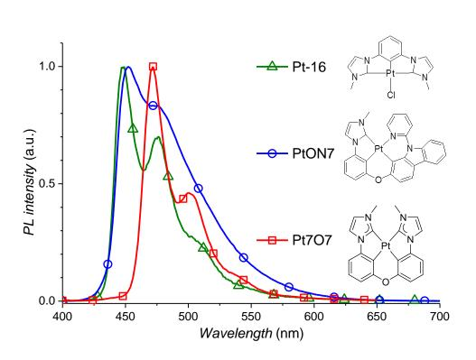
Following the materials design principle from tetradentate Pt complexes, Pt7O7 was synthesized and fabricated in the device settings. We were very thrilled to report that the monomer and excimer can both be efficient at the same time with peak EQE close to 25% and peak power efficiency close to 60 lm/W.
