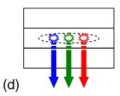
Schemes for 4 possible WOLED architectures: (a) triple-doped emissive layer; (b) multiple emissive layers; (c) emissive layer with monomer and excimer; (d) emissive layer with a single broadband emitter.
