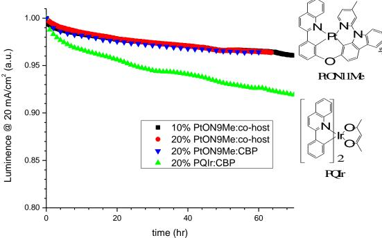
PtON11-Me, a analog to PtON1 and PtON7, have demonstrated a remarkable operational stability in OLEDs. The LT<sub>97</sub> is more than 70 hrs at a very high current density of 20 mA/cm<sup>2</sup>, indicating the potential of such class of emitters as emitters for the stable and efficient blue and white phosphorescent OLEDs.
