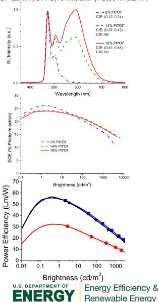
ITO/HATCN(10 nm)/NPD(30 nm)/ 14% Pt7O7:mCBP (25 nm)/BAlq(10 nm)/Alq3(30 nm)/LiF/Al.
