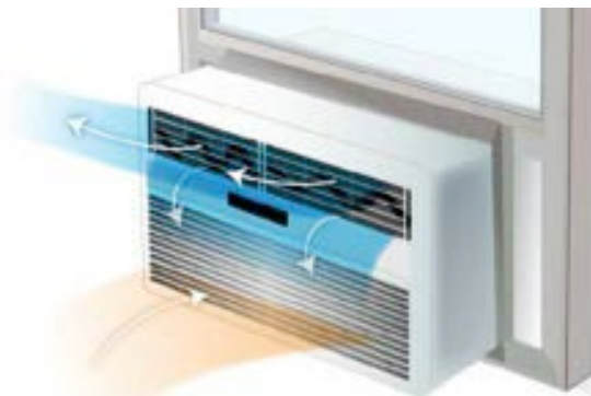
One problem with window air conditioners is that a significant portion of the conditioned air gets recirculated back into the air conditioner.
