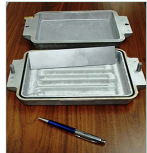
Figure 1-3. Clamshell with fuel plate
