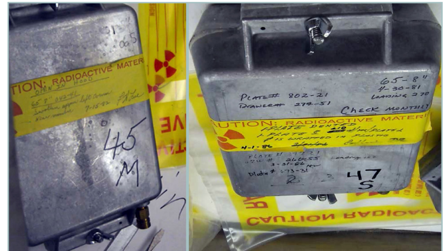
Figure 1-4. Clamshell 45 M (left) with notes that upper left corner of fuel plate is open and to open in hood and Clamshell 47 S (right) with notes that plate is dented and wrapped in plastic and the direction to check monthly
