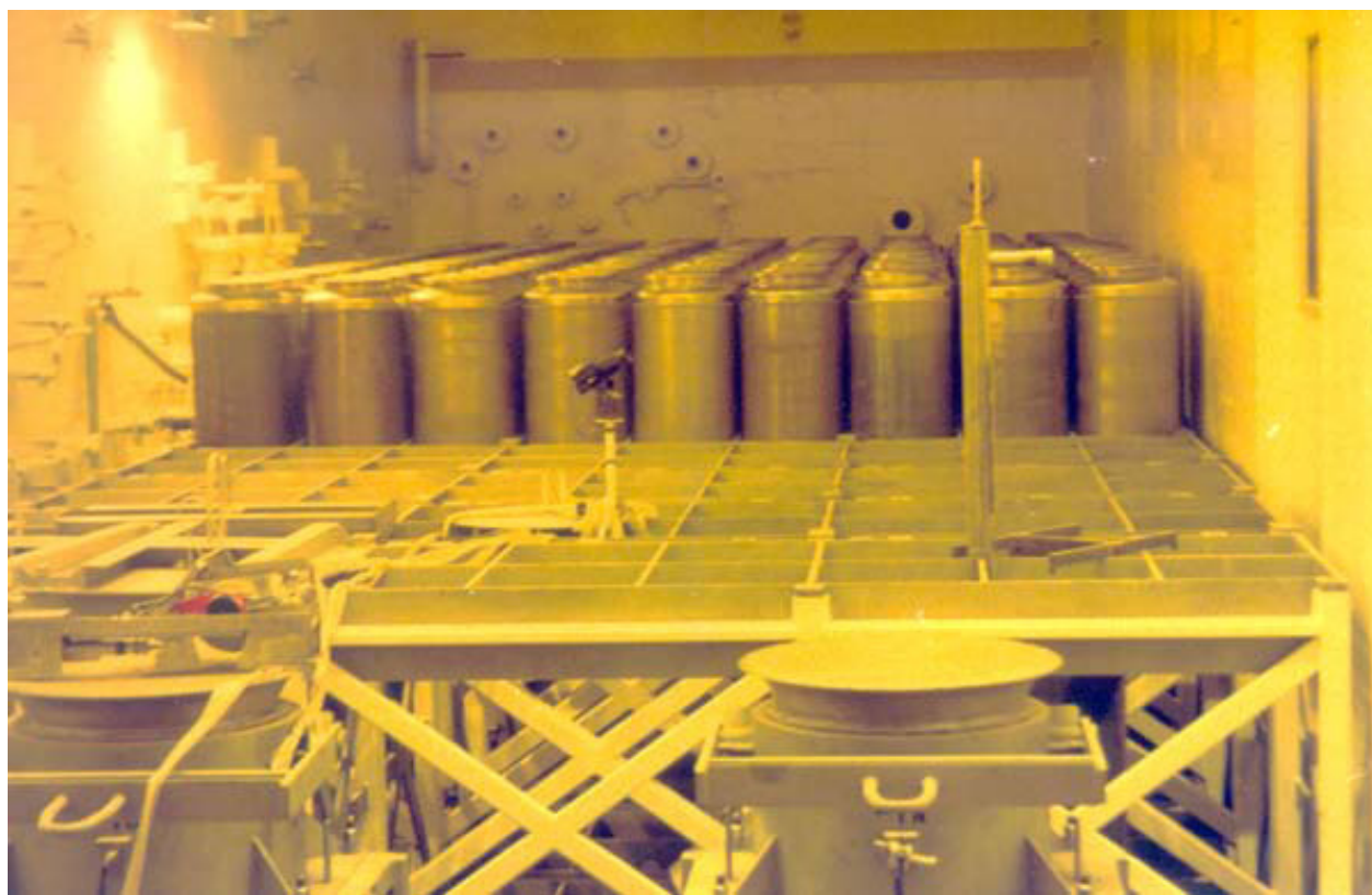
Figure A-17. Photograph of HLW glass canisters stored in the chemical process cell of WVDP main process building
