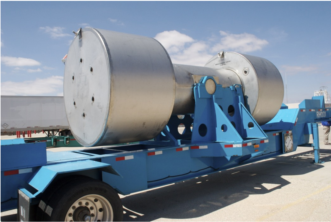
Figure B-8. Photograph of RH-72B waste transport system
