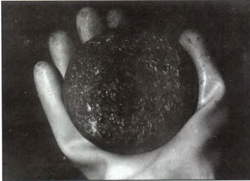
Plutonium Button and Rubber Glove, Rocky Flats Plant, Colorado, 1974. Virtually everything involved in plutonium processing, such as this rubber glove, becomes contaminated and must be contained and monitored indefinitely. This waste is called "transuranic" waste, which includes any material containing significant quantities of plutonium, americium, or other elements whose atomic weights exceed those of uranium. Transuranic waste can include everything from chemicals used in plutonium metallurgy to used air filters, gloves (see photo), clothing, tools, piping, and contaminated soils.
