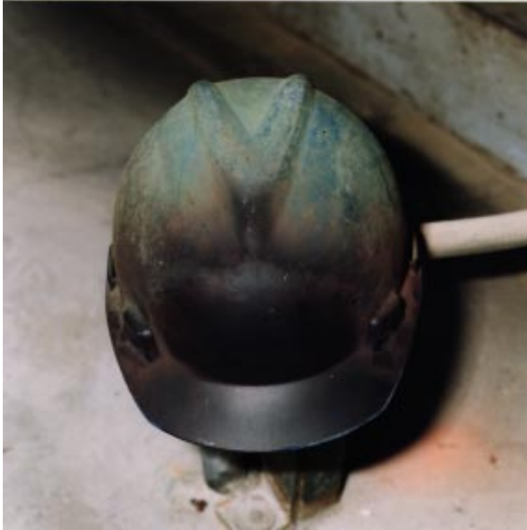
Exhibit 2-4. Electrician B's Hard Hat After Electrical Arc Blast
