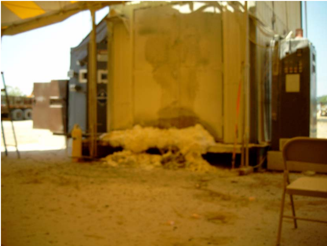
Figure 2-6. Remnants of the Exothermic Sodium Reaction
