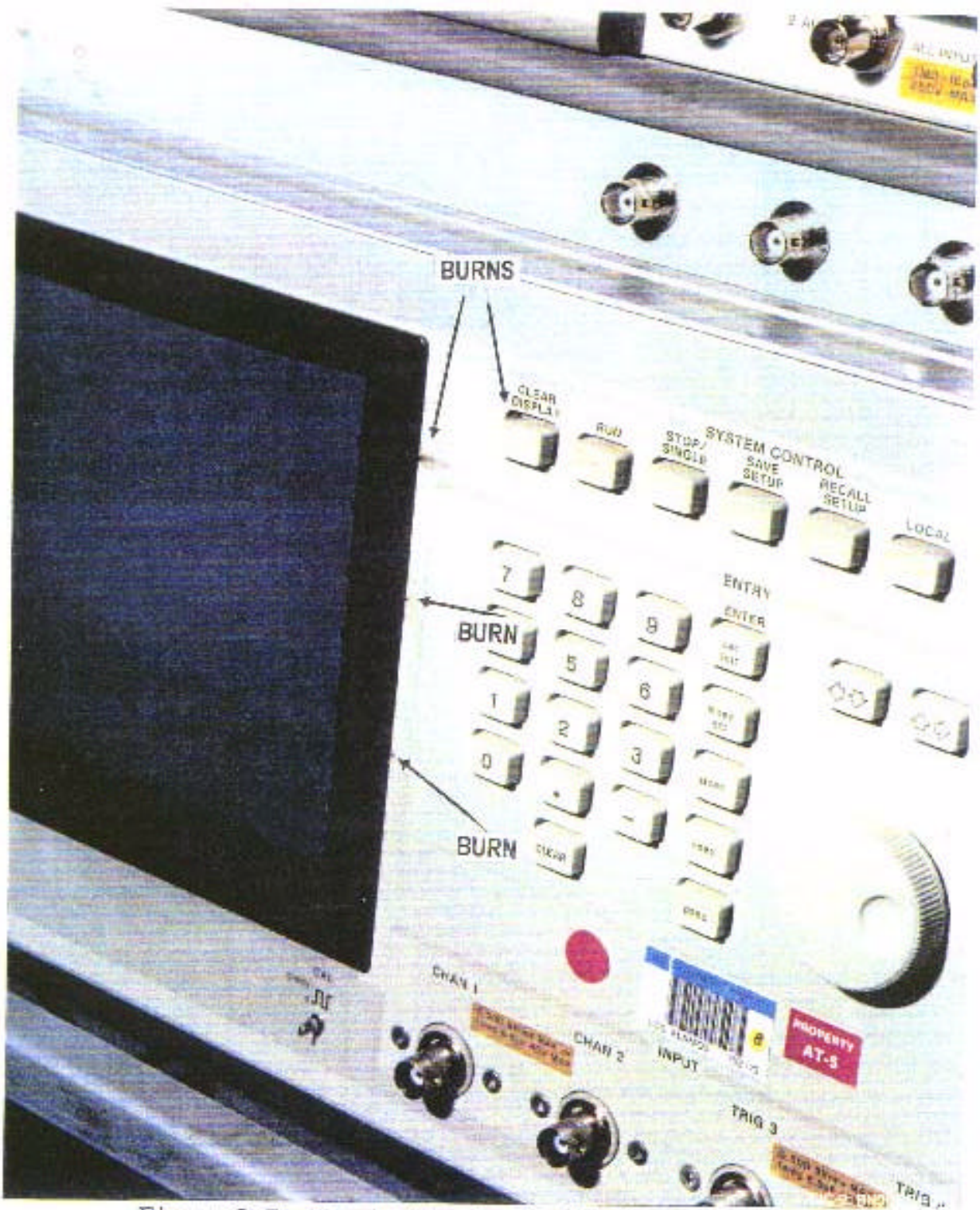
Figure 2-7: Hewlett Packard 54111D Oscilloscope Showing Burn Marks
