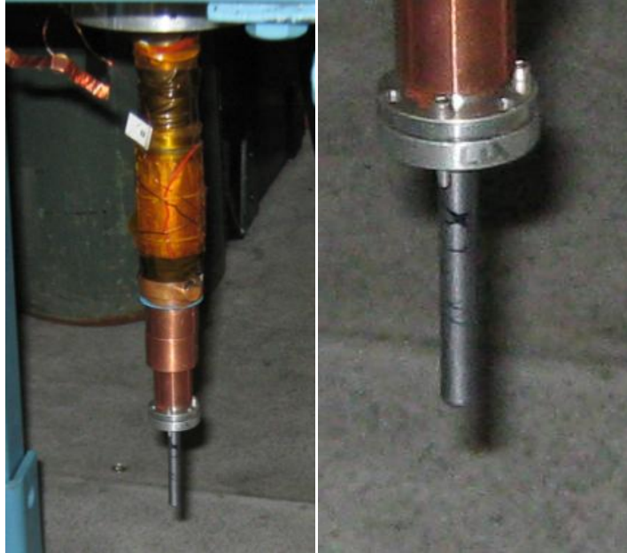
Figure 2.1.7. Displex Cold Finger and Close Up of Tungsten Sample
