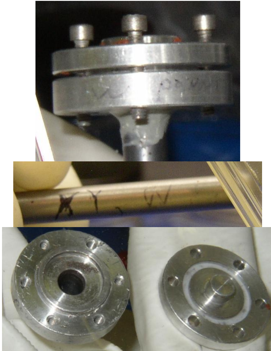
Figure 2.1.14. Lutetium Technetate Canister Re-used for W (Tungsten)
