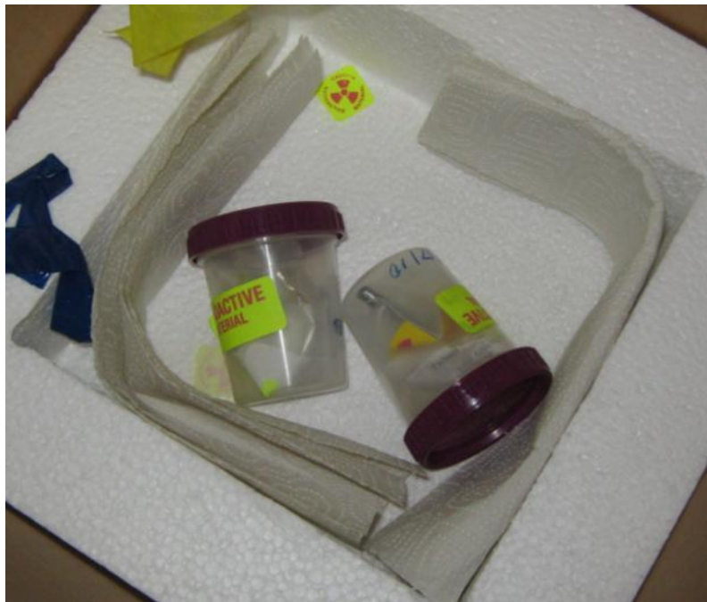
Figure 2.1.5. Pr and Nd Technetate Sample Canisters
