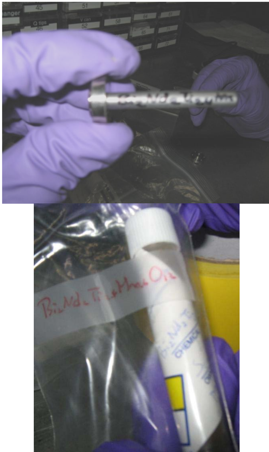
Figure 2.1.11. Empty Vanadium Tube and Collar from Sample Desk with Zip-lock Bag and User Sample Staged for Processing
