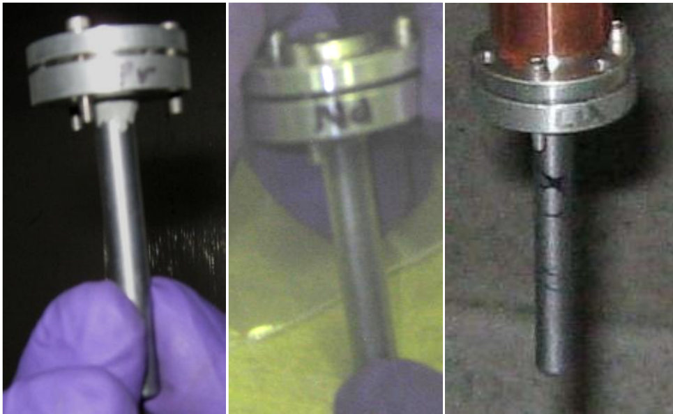
Figure 2.1.13. Comparison of Pr, Nd, and Lu/W Sample Canisters
