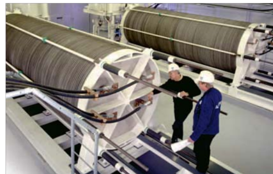
The atmospheric series Norsk alkaline electrolyzers with a unit production capacity of 1000 kg/day, with larger volumes produced by stacking multiple units http://www.electrolysers.com/
