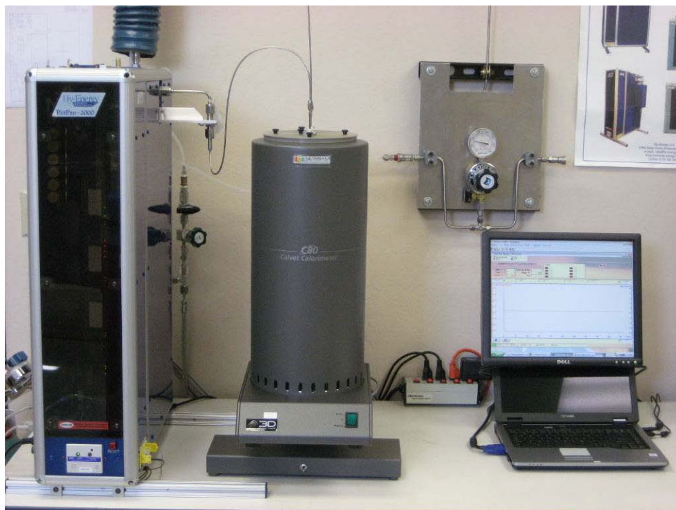
Figure 224. PCTPro-2000 Sievert's apparatus coupled with a C80 calorimeter permitting simultaneous measurements of gas adsorption/desorption and heats of sorption. 303
