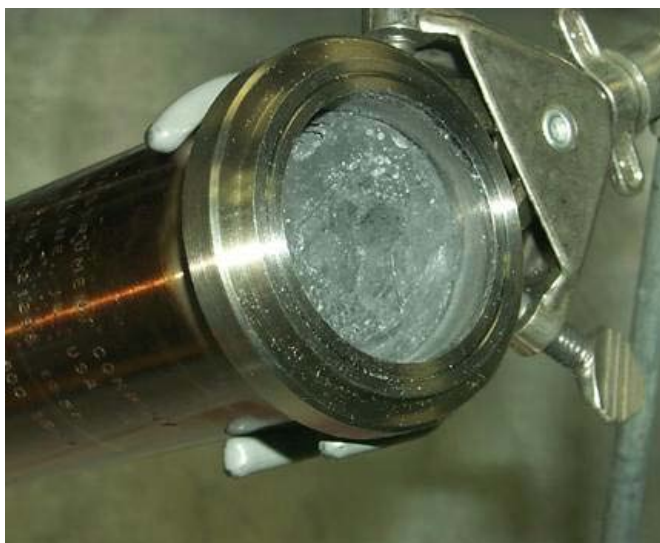
Figure 233. Scale up (100 g) reactor with end cap removed in Ar-glovebox to show catalyzed alanate. 121
