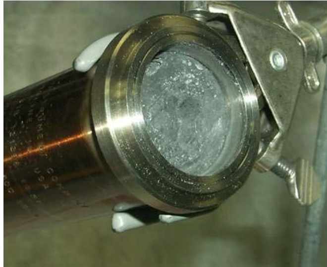
Figure 48. Scale up (100 g) reactor with end cap removed in Ar-glovebox to show catalyzed alanate. 121
