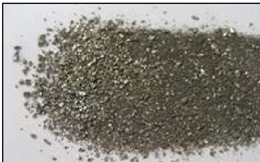
Figure 227. After 32 cycles LaNi 5 sample still contains 5/6 of a course un-reacted material. 303
