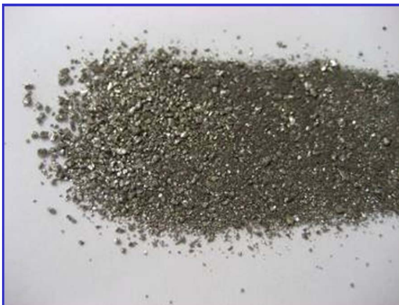
Figure 119. Photo of incompletely hydrided \text{LaNi}_5 . 177
