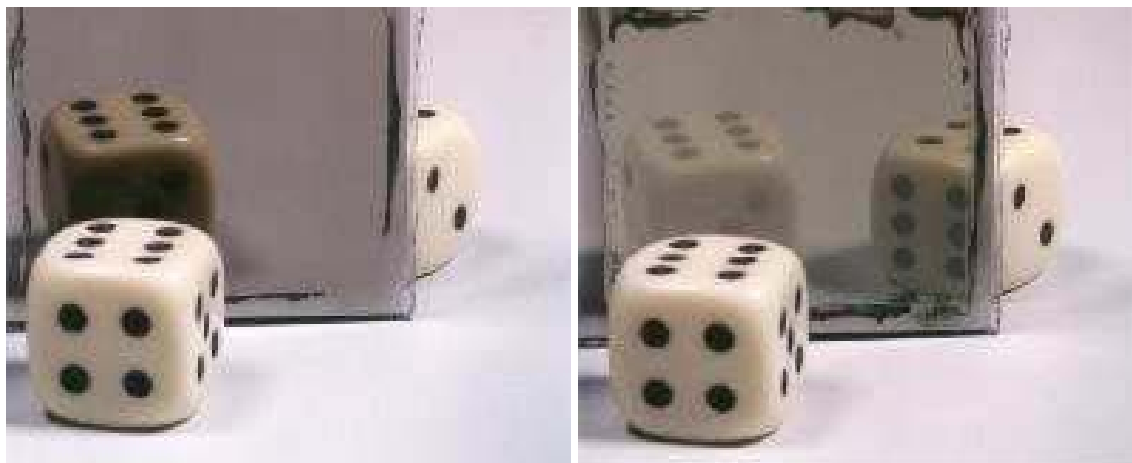
Figure 217. Metal hydride thin film in the metallic (left) and in the hydrided (right) state during electrochemical loading. 292
