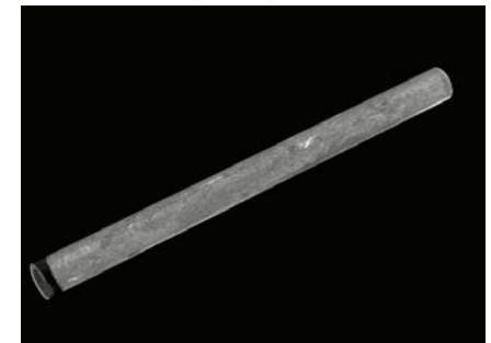
3D CT Scan of field-generated foamed cement. Foam quality 47.8%; collected at a pressure of ~290 psi
