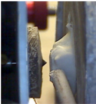
Figure 1. Photograph of micro-indenter in operation.
