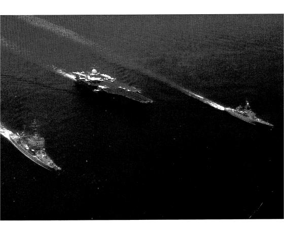
**36.** The nuclear-powered aircraft carrier *Enterprise* (CVAN-65) in action. The tremendous power of her eight-reactor propulsion system is dramatically demonstrated in this high-speed turn. *U.S. Navy*
