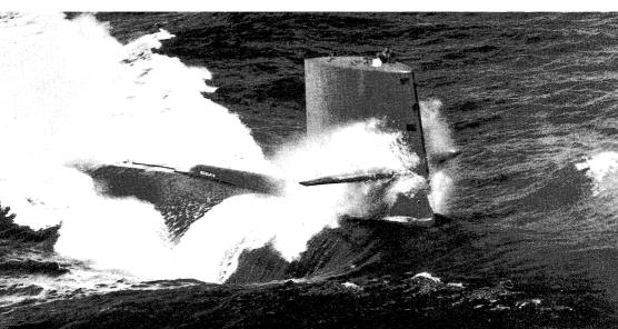
**33.** The *Triton* (SSRN-586) leaving New London on February 16, 1960, for a trip around the world. Driven by two S4G reactors, the largest submarine ever built circumnavigated the globe, submerged, in 83 days and 10 hours.
