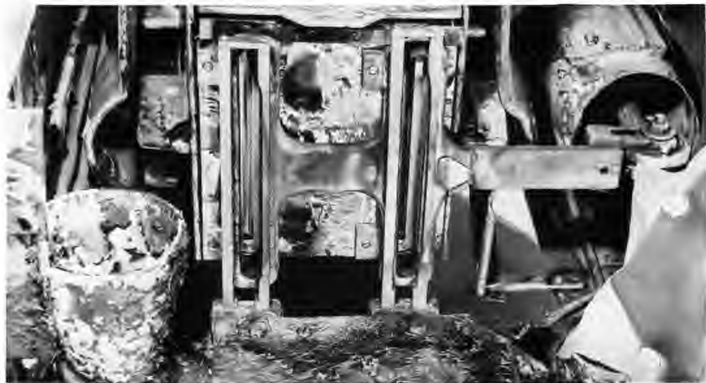
BETA SOURCE UNIT / During operation the two beams of ions were projected from the vertical slots. At the conclusion of a run it was necessary to wash off and recover the uranium tetrachloride scale.
