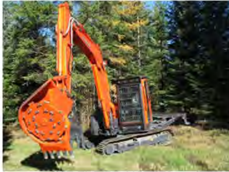
18,000# Kubota excavator with Advanced Forest Equipment mulching head
