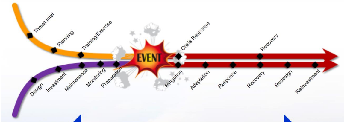
Figure 2. Critical Infrastructure Planning and Operations Timelines: The top-most vector represents operator knowledge and actions. The bottom-most vector represents various aspects of system design and operation.
