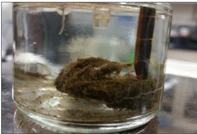
Algae biofilms accumulated on glass washers affixed to a plastic pegboard submerged in East Fork Poplar Creek. ORNL researchers analyzed the samples to determine the production of methylmercury.
