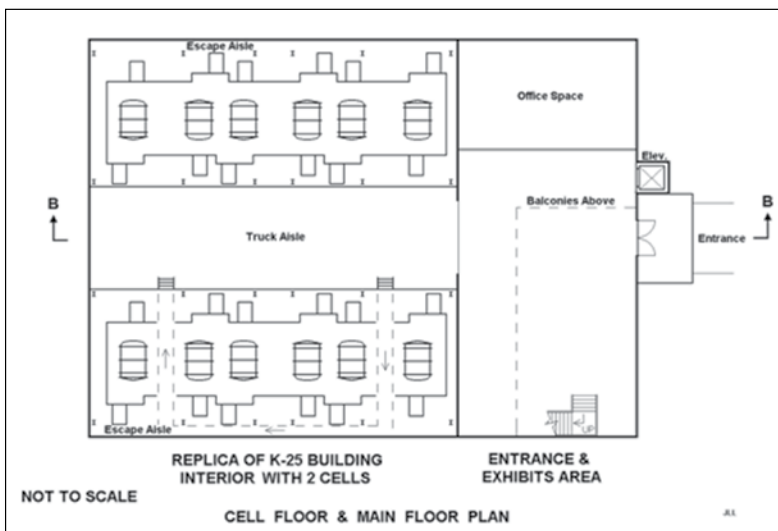
A floor plan of Concept B, which would be a replica of the North Tower of the K-25 Building.
