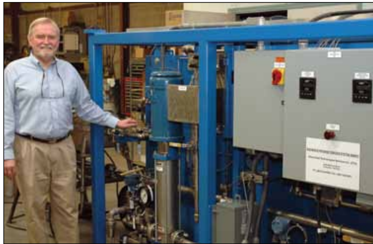
ORSSAB member Chuck Jensen stands beside a Radwaste Reverse Osmosis System that his company, DTS, manufactures to remove radioactive isotopes from contaminated water.
