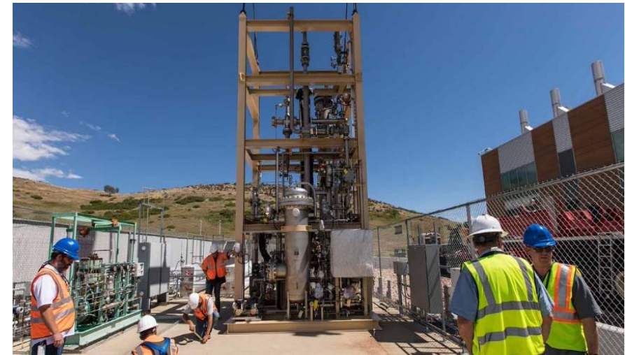
Water Electrolysis & Biomethanation demonstration at NREL (Golden, CO), 700 liter vertical, stirred bioreactor.
