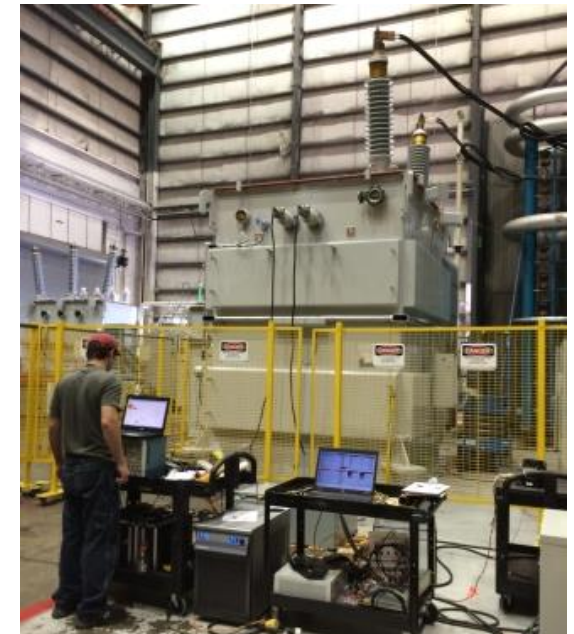
Transmission level CVSR prototype from previous ARPA-e project
