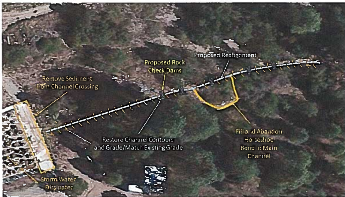
Figure 3. Channel Stabilization Project Map. This project will stabilize the main channel directly downstream of the dissipation structure, straighten the channel and fill in the sharp bend, line the bank and channel bottom with TRM, and install 4-5 rock check dams.
