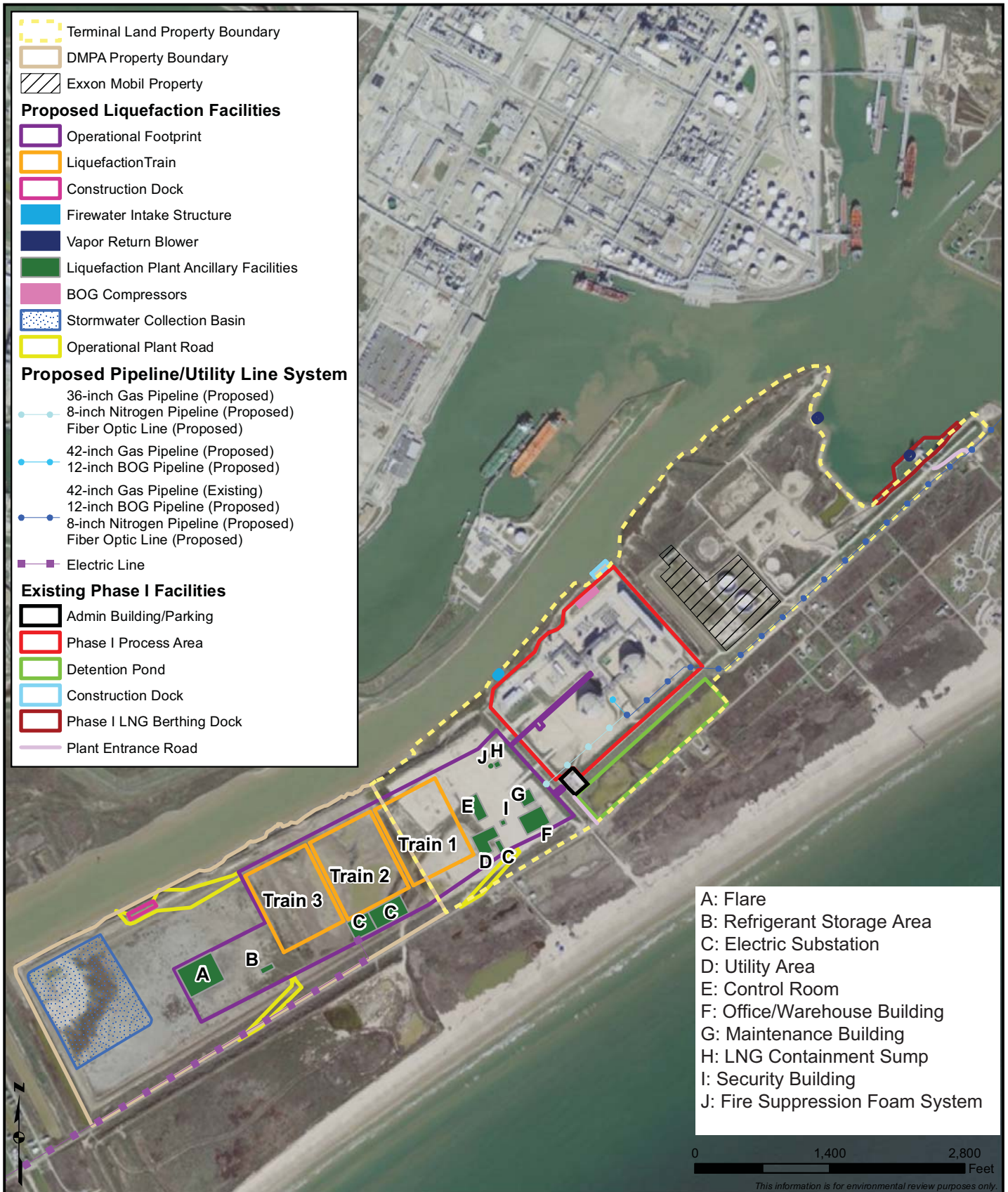
Figure 3.3.1-2 Freeport LNG - Liquefaction Project Proposed Liquefaction Facilities at and Adjacent to Quintana Island Terminal Brazoria County, Texas
