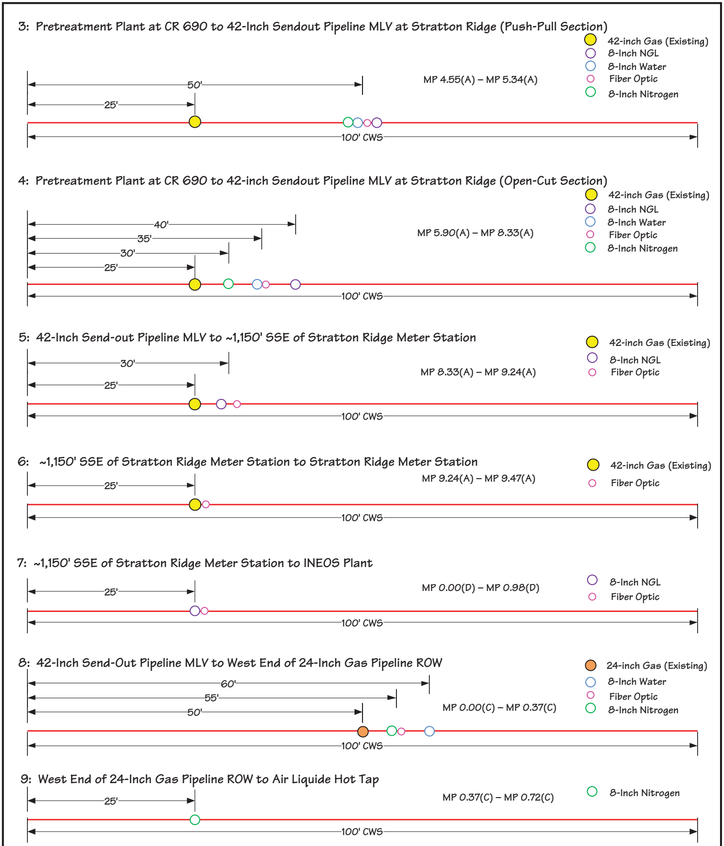
Figure 2.4.1-2 Freeport LNG – Liquefaction Project Construction Right-of-Way Cross-Sections for Non-Jurisdictional Pipelines/Utility Lines North of Pretreatment Plant
