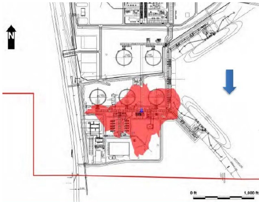
Figure 7: Time Composite Image of Vapor Dispersion for the 2-inch hole Release from the Tank Sendout Header with Wind from the North (Scenario 3).
