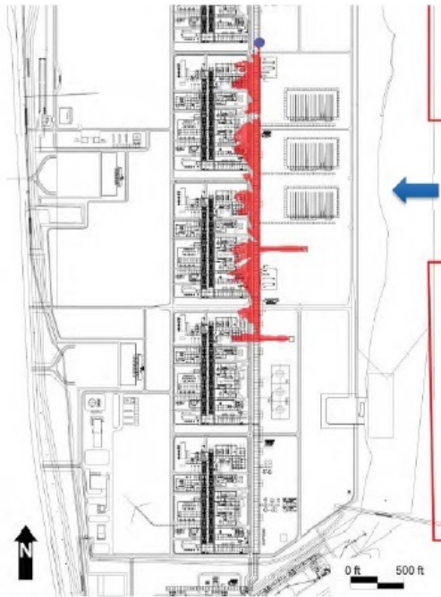
Figure 9: Time Composite Image of Vapor Dispersion for the Guillotine Release from the LNG Rundown Header at Liquefaction Trains 4 and 5 (Scenario 4) with Wind from the East.
