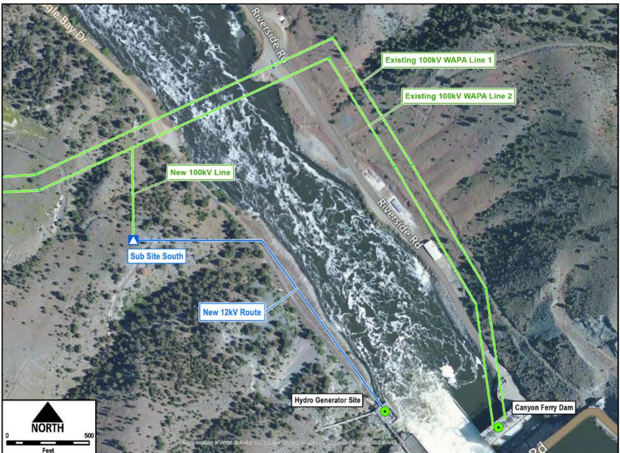
Figure 10. Alternative - Distribution Line and Substation.
