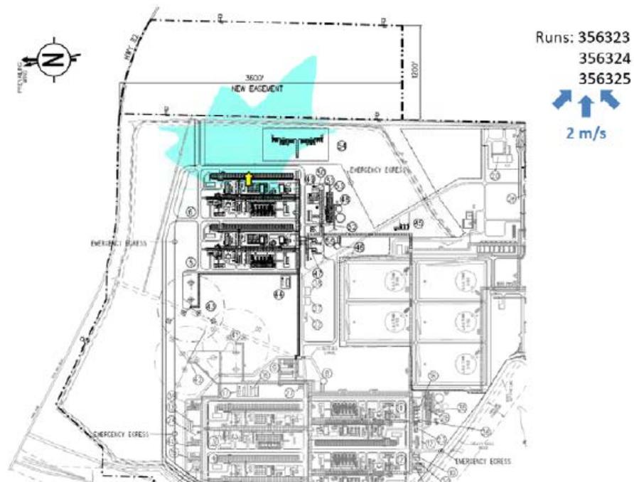
Figure 4 Propane Vapor Dispersion Zone – Flashing and Jetting
