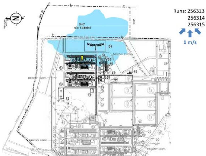
Figure 3 Ethylene Vapor Dispersion Zone – Flashing and Jetting
