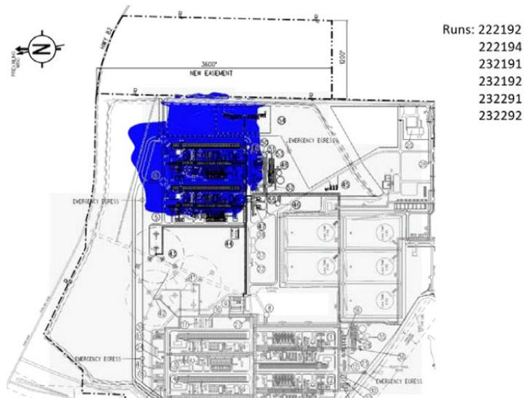
**Figure 5 Extent of 1 Psi Overpressures due to Ethylene Design Spill in Train 6 – Shown as Shaded Areas**
