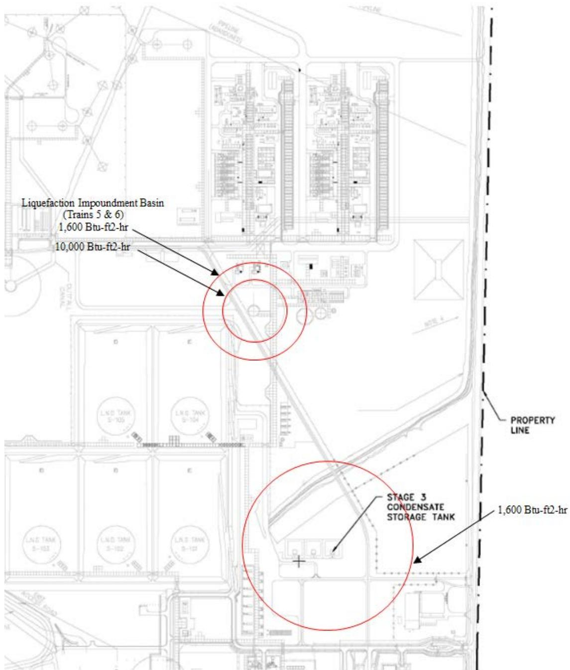
**Figure 6 Thermal Radiation Distances (1,600 Btu-ft<sup>2</sup>-hr) for the LNG Impoundment Basin (Trains 5 & 6) and Condensate Storage Tank Area**
