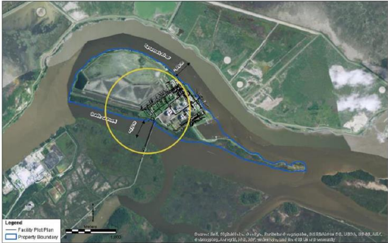
Figure 2.8.6-4 – Jetting and Flashing Scenario from the LNG Rundown Line at MMLS Unit Closest to the Property Line Adjacent to the South Channel
