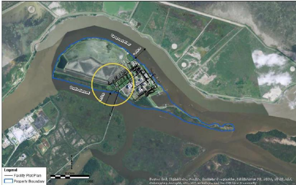
Figure 2.8.6-6 – Jetting and Flashing Scenario from the LNG Rundown Line at MMLS Unit Closest to the Property Line Adjacent to the South Channel Modeled with Two Check Valves
