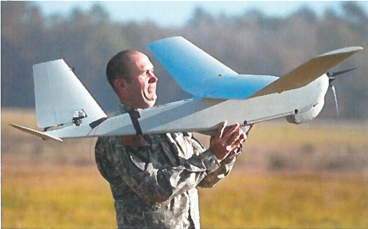
Figure 2. Puma RQ-20A fixed-wing unmanned aircraft
