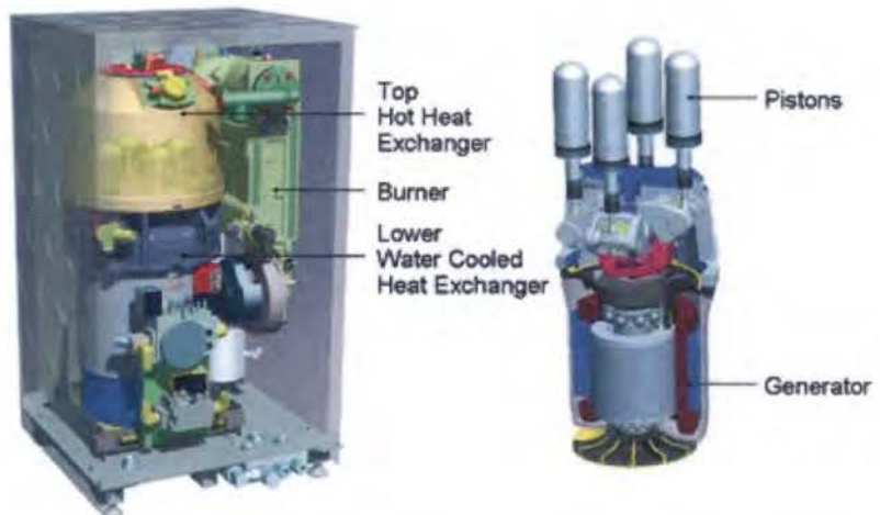
Sectional views of the four cylinder Stirling engine heat and power system. (Figures courtesy of WhisperGen Ltd.)
