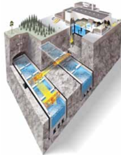
Sweden's centralized interim storage facility for UNF has been in operation since 1985. The underground portion (illustrated below) comprises two rock caverns with eight storage pools.
